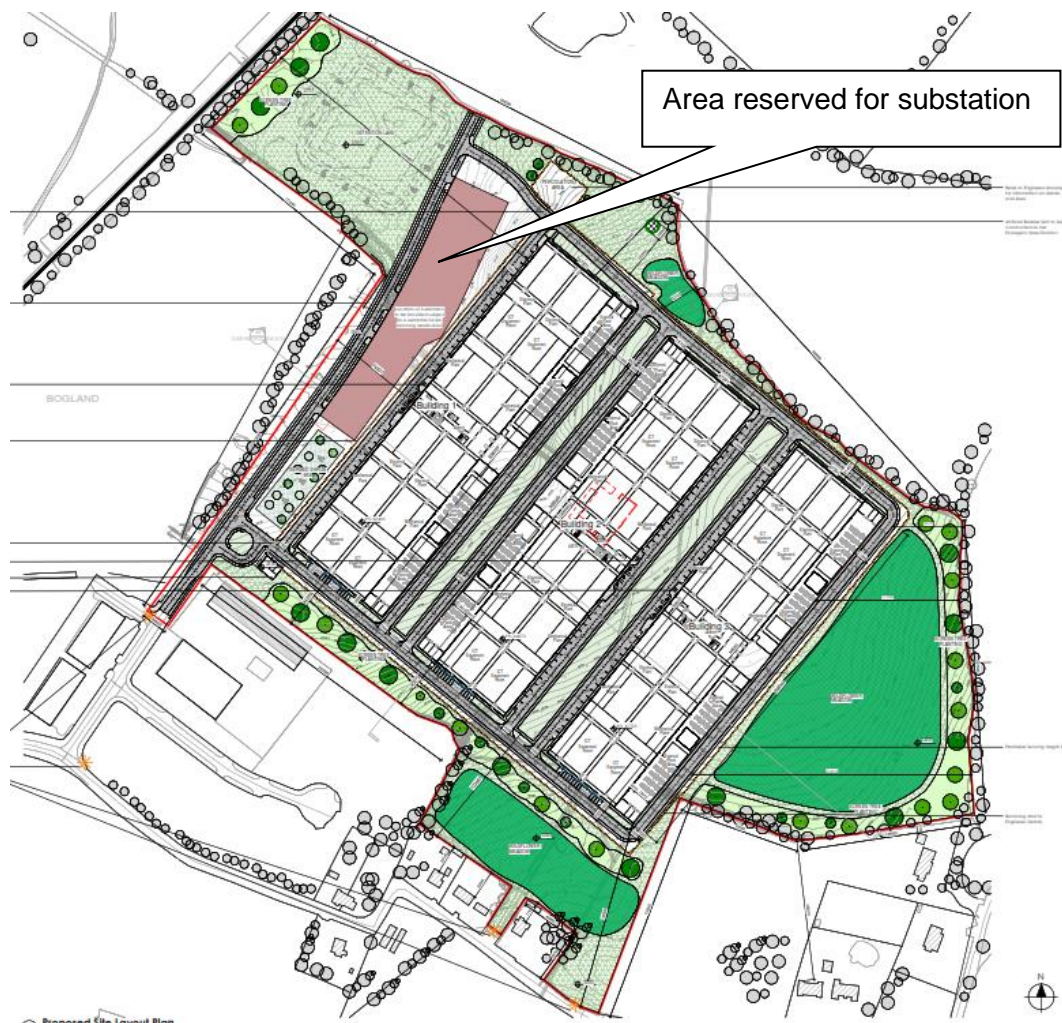
Figure 3.1: Extract from the site layout plan from application Reg. Ref.: 20/1088, labelled to indicate the location reserved for the substation now proposed
